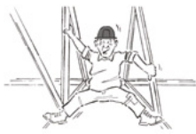
Trusses DO need bracing
