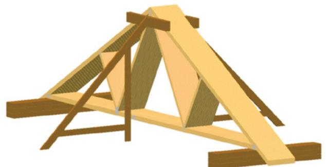
When trusses are stored horizontally level bearers should be positioned beneath each truss node as a minimum. (Fig. 2). Other methods of storing trussed rafters may cause deformation and distortion unless specific provision has been made in the design for an alternative temporary support load case.
